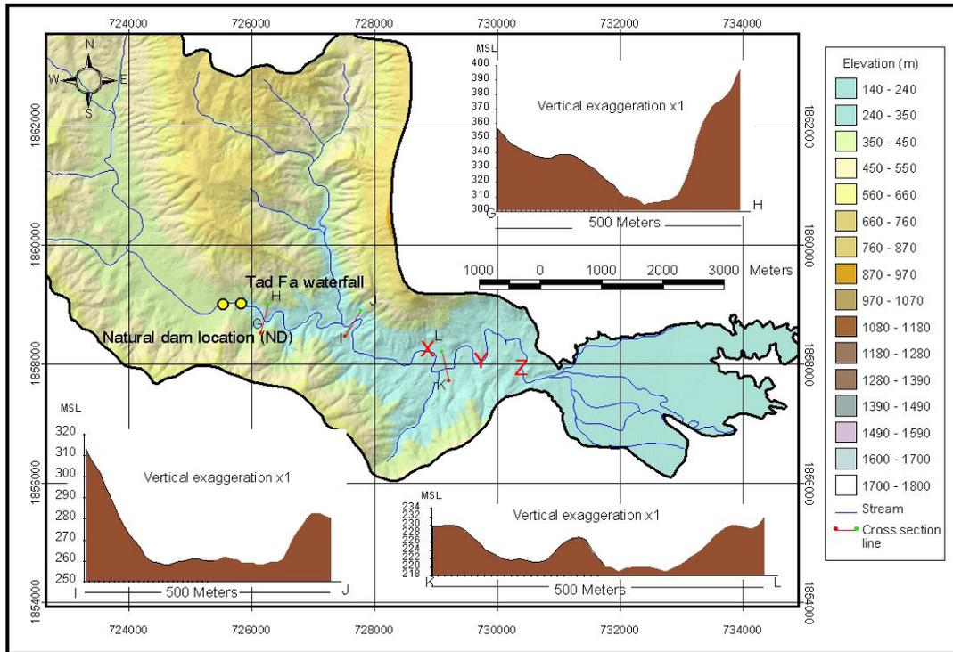
Figure 5-11 Three cross-sections (line G-H, I-J and K-L) across Nam Ko Yai stream channel and its valley at the downstream areas from the suspected natural landslide dam location (ND).
