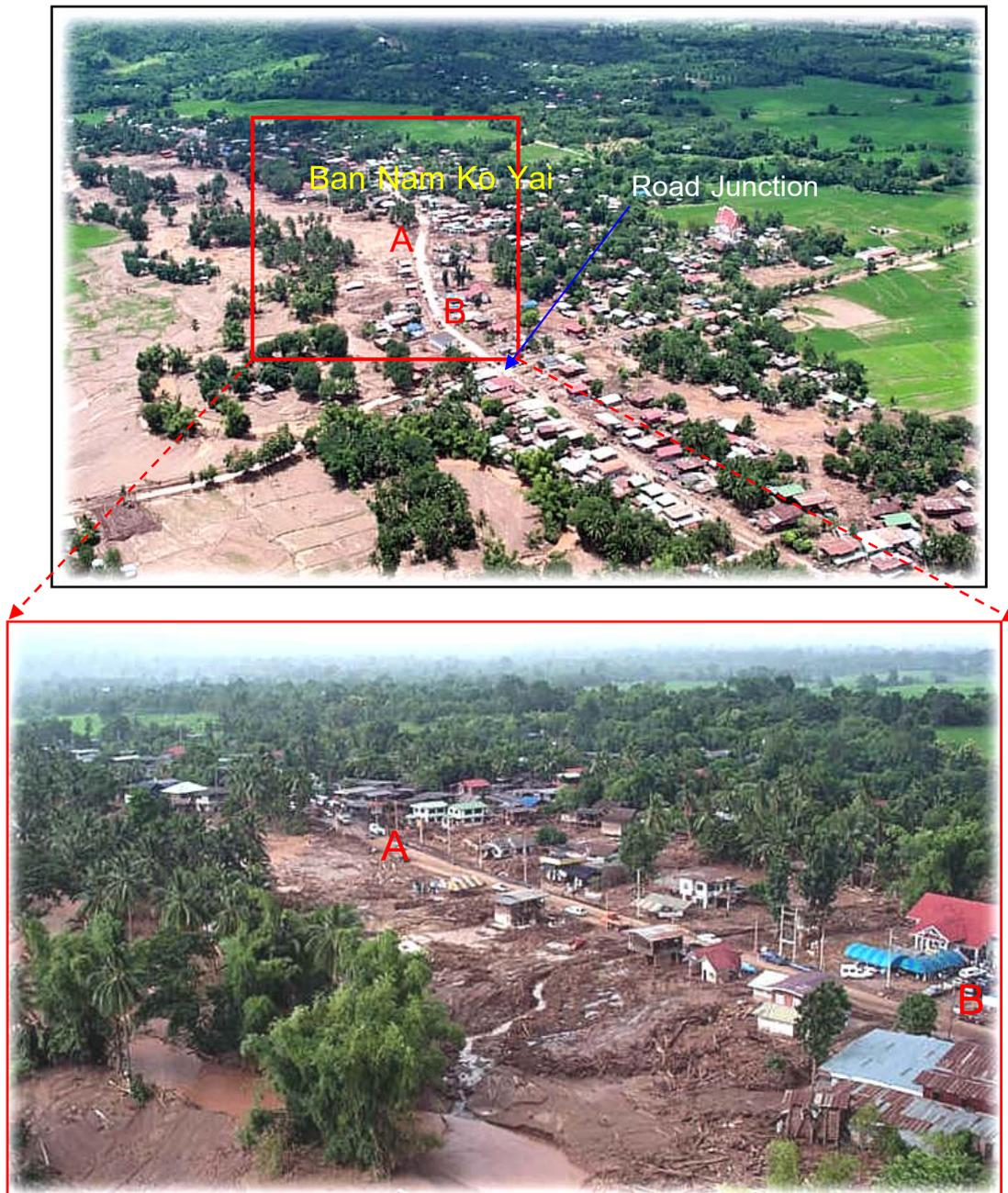
Figure 6-5 Two oblique aerial photographs perceptibly illustrating the characteristics and extension of a large volume of deposited sediments as evidences of 8/11 incidence.
