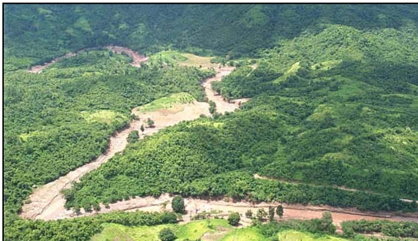
Fig. 14 The oblique aerial photograph (taken on 22 August 2001, 11 days after the event) along the channel of Nam Ko Yai stream with the high sinuosity characteristic illustrating the debris flow-flood track along plant debris and soils had been strongly eroded and transported from its banks before reaching the canyon mouth outlet of the stream
