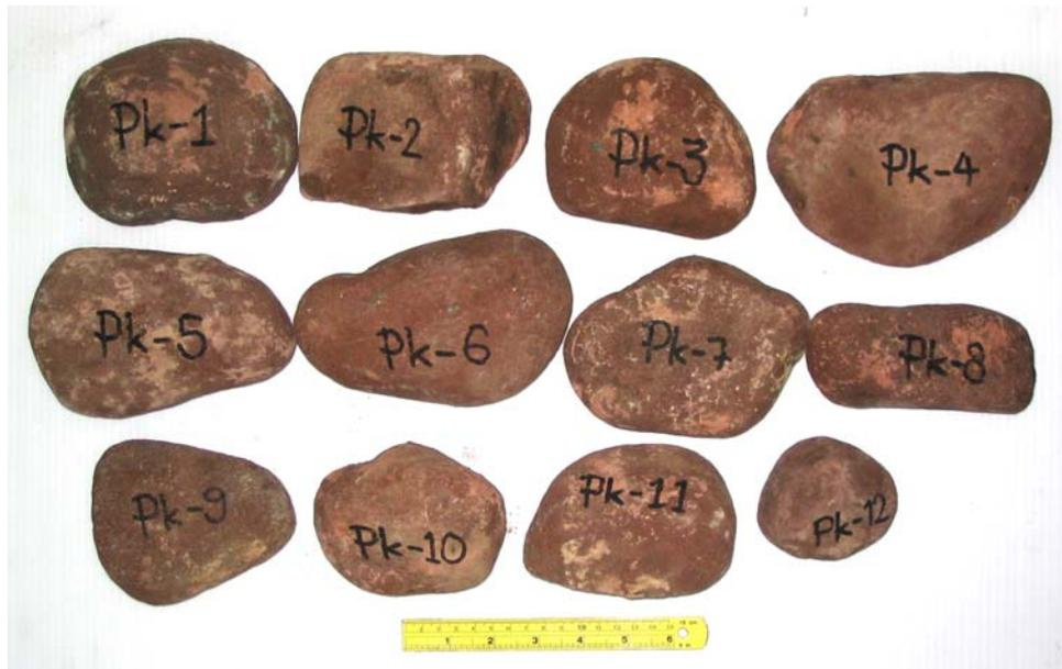
Appendix B-8 Characteristics of twelve rock specimens of Phu Kradung sandstone/siltstone (lithologic unit Pk) after point load testing
