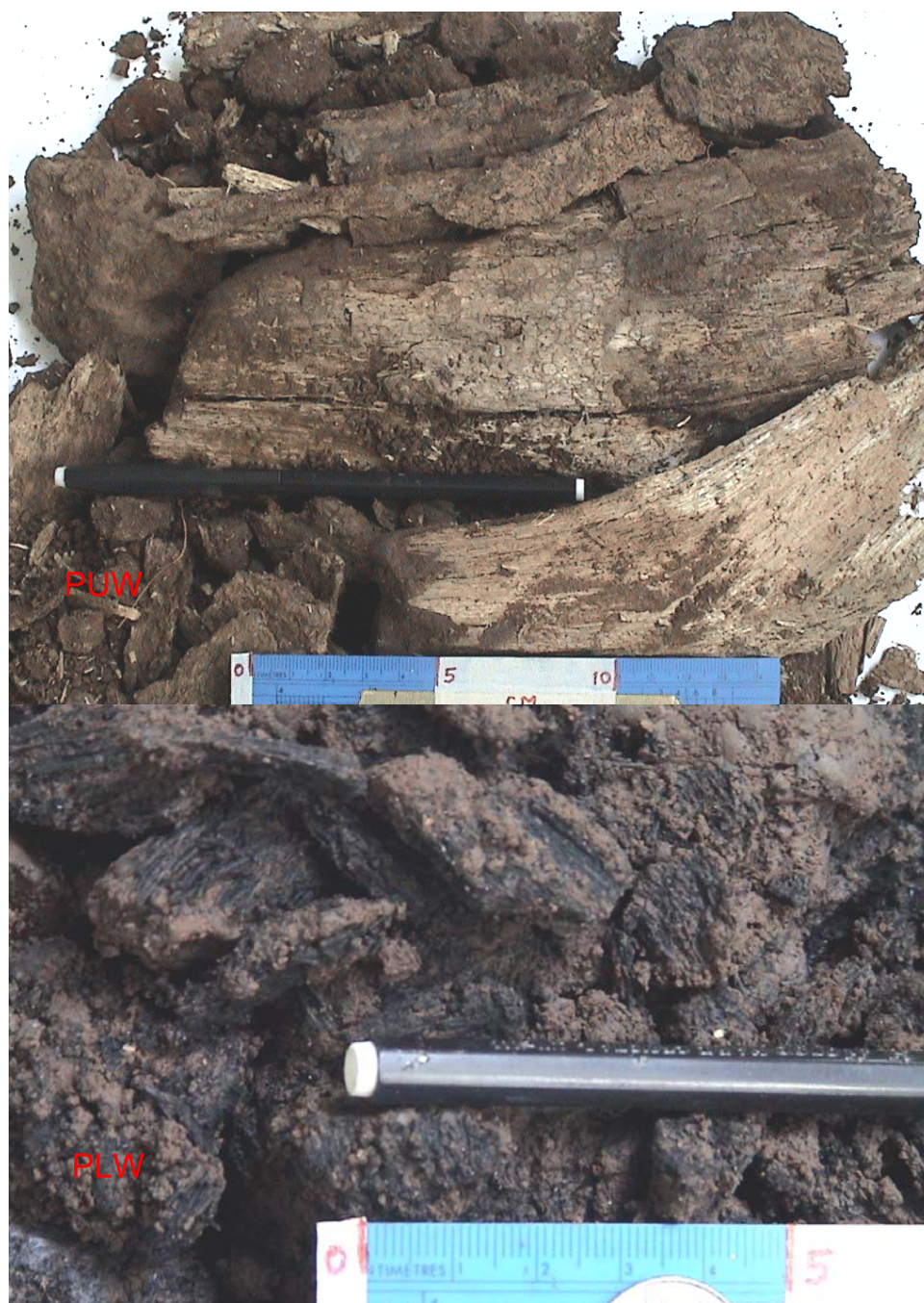
Figure 6-17 Closed-up photographs of the collected wood debris samples from the preserved locations at PLW and PUW (as shown in Figure 6-16) illustrating their general characteristics of charcoal characteristic with fibrous texture and pale brown wood with rather complete wooden texture, respectively.
